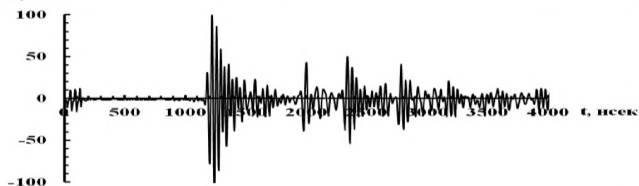
Fig. 6. The window illustration of data treatment of quasilongitudinal elastic waves velocity measuring V_{\parallel} = 2485 \pm 10 m/sec in porous polystyrene C_8H_8 by impulse-phase method at frequency f_{\parallel} = 1 MGz.
