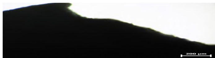
Fig. 2. Microstructure of surface irregularities h = 22 \pm 11 mkm of initial zeolite mineral \text{Ca}[\text{Al}_2\text{Si}_4\text{O}_{12}]x2\text{H}_2\text{O} before loading at filter.
